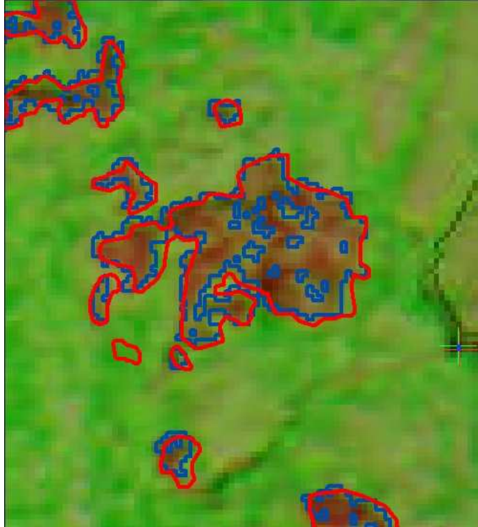
Figure 7 - Automatic detection (blue) plotted against reference data (red) superposed to MODIS imagery [4]
